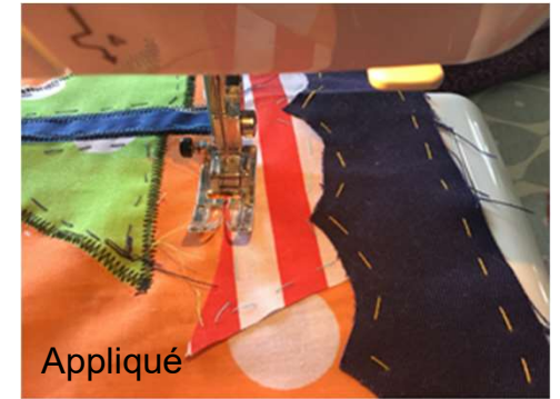
Tacking is temporary hand sewing stitch to hold fabrics together
